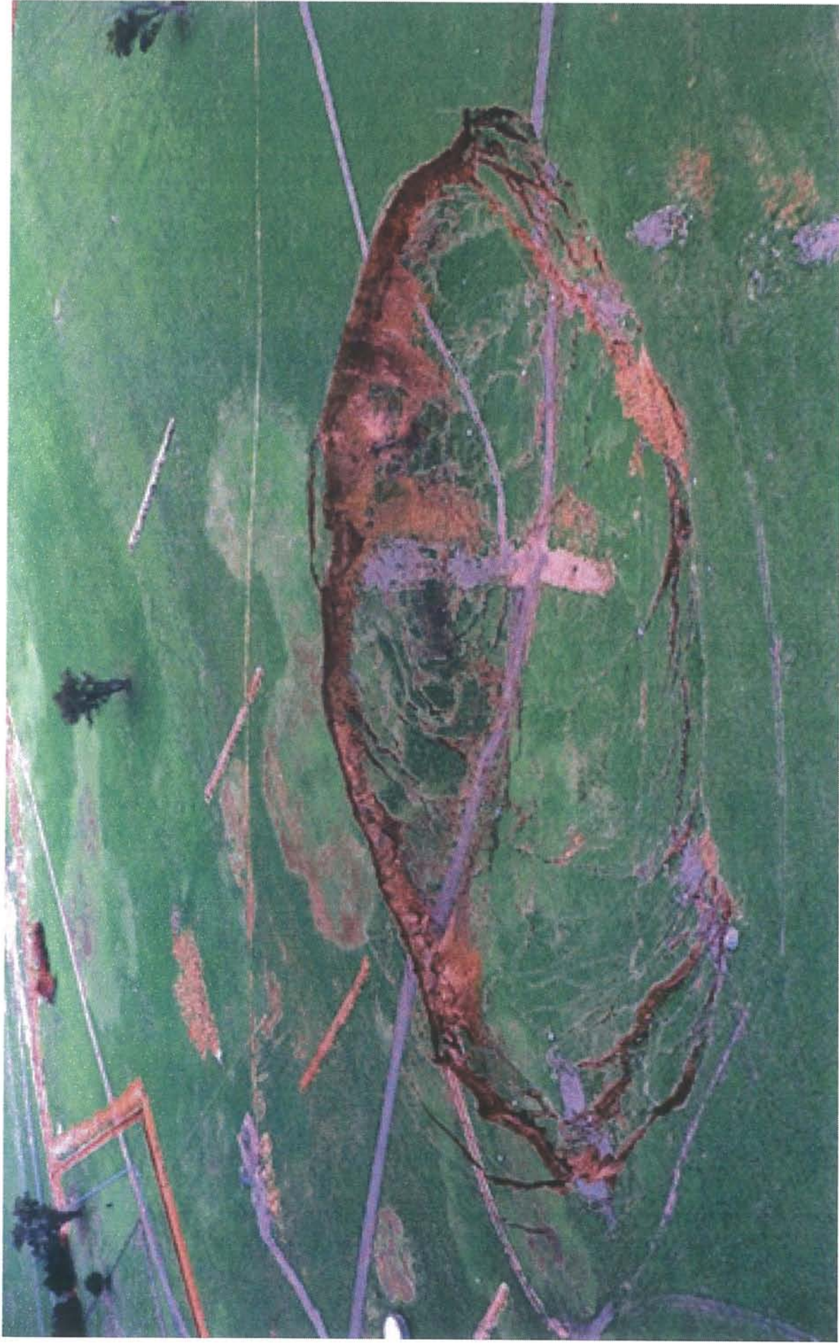
Subsidence from Block Cave Mining at the Ridgeway Mine in New South Wales, Australia http://www.pebblescience.org/Pebble-Mine/block_caving.html
