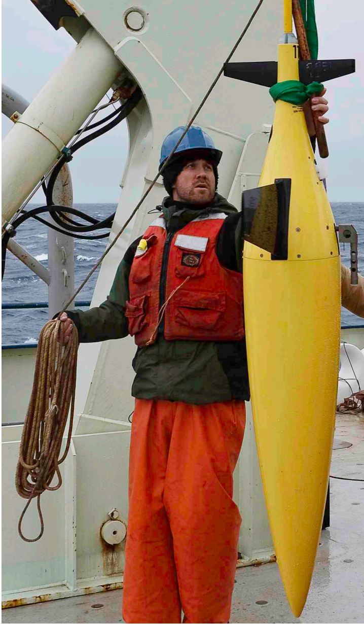
Figure 6. Sea glider tested under sea ice in the Davis Strait. Robotic instruments like these are making observations under ice that were previously impossible to gather. Photo courtesy of Craig Lee.
