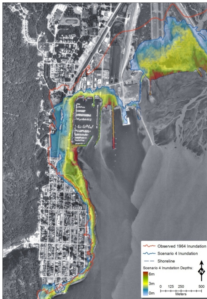
Tsunami inundation scenario for Seward. Such maps are the foundation for tsunami evacuation planning and for the siting of emergency facilities. This work is performed at UAF and supported largely under the authorization of TWERA.
